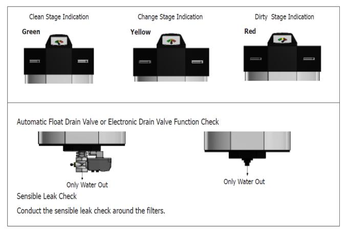
2.During the change Signal we need to prepare for the filter element change. The filter element must be changed at change stage indication.
