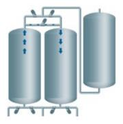
3. Next, the pressure between the two cylinders is equalized.
